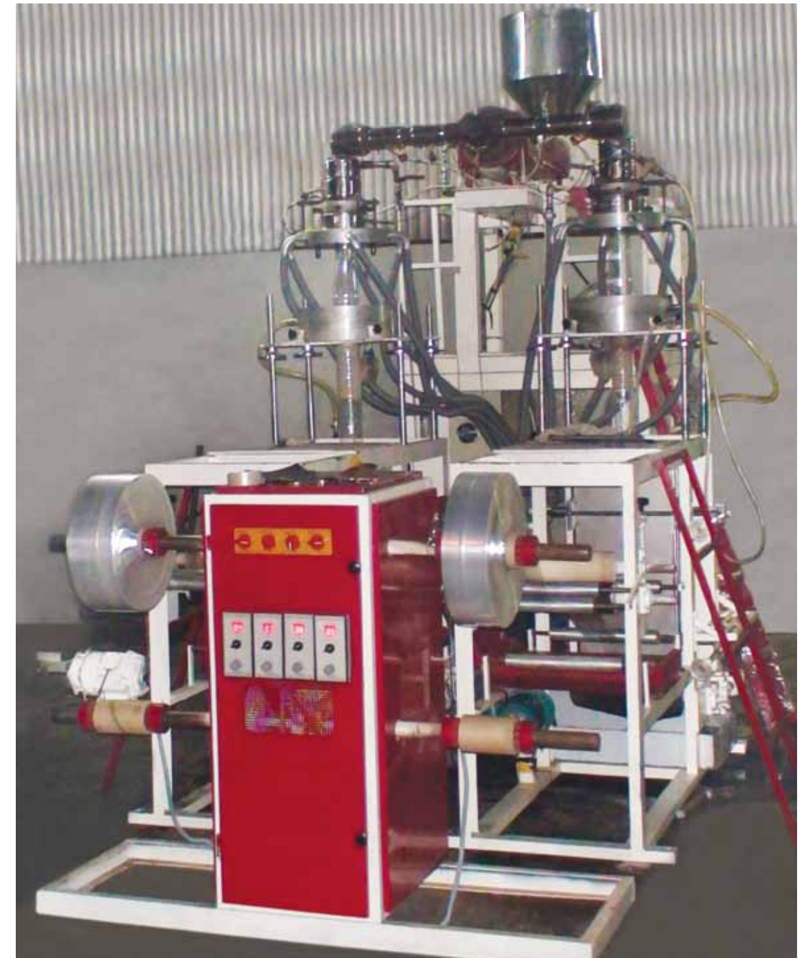
RK TWIN DIE PP BLOWN FILM PLANT
