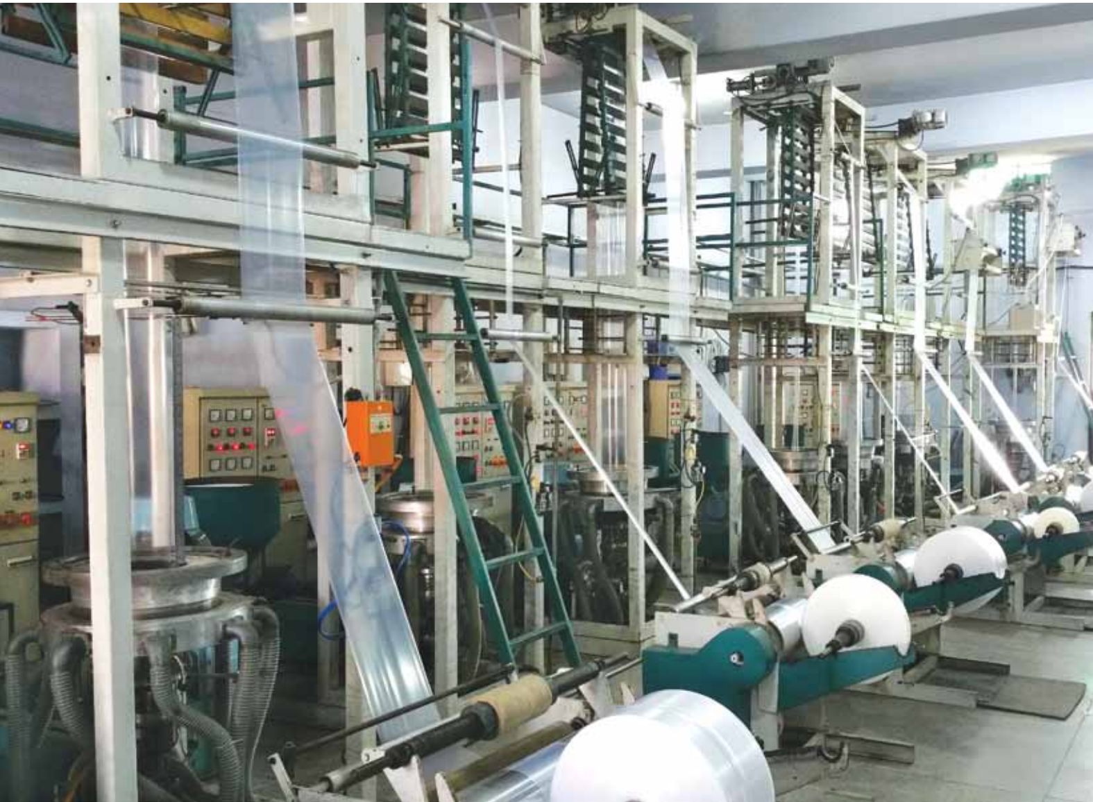
RK LDPE HDPE BLOWN FILM PLANT
