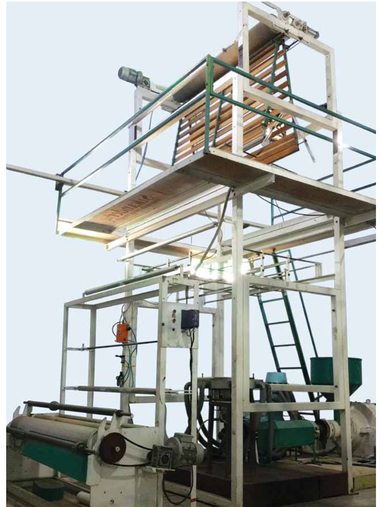
RK 55-75MM LDPE HDPE FILM PLANT
